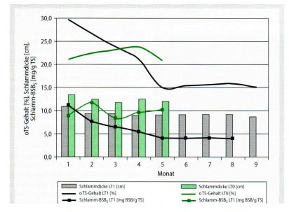
Laboratory pond: course of sludge parameters (sludge BOD5, oTS content, sludge thickness) in LTO and LTI during the study period; no degradation of sludge parameters occurred without aeration (LTO). In the aerated laboratory pond (LTI), however, there was a significant degradation of the sludge parameters.
