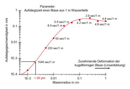
Fig.7 Ascent velocity of a bubble depending on the bubble radius.
